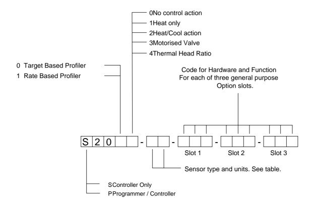
Example 1. S2001-03-4BB-3II-1GH This describes a controller only, with a heat only analogue control. Input via a type K thermocouple working in degrees C. The option slots configured as follows:-
