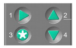
The essence of the password is a four digit code representing a sequence of four button presses. When the password is being entered any of the four front panel buttons are valid, they are arbitrarily assigned values 1 to 4 with the scroll button as 1 etc.
