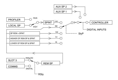
The Series 2000 instrument may have many different setpoint sources for its internal controller. Setpoints may be input from external devices in either digital or analogue form and combined with the internal setpoints in various ways before being passed to the controller.
