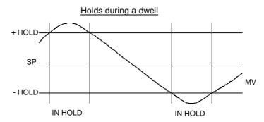
Dwell timer suspended during hold. Note that 'Above', 'Below' and 'Dwell' holds at least are set on in the hold-type parameter of the programmer long scroll.
