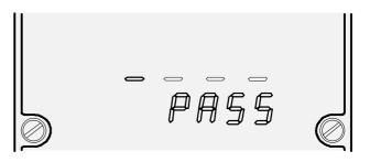
on the correct password being entered, and then enter the appropriate long scroll. Unless the password is correctly entered, protected parameters can be viewed but not modified.
