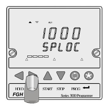
user will scroll to the required group and then press the star button to enter the group. Further presses of the scroll key will then access the individual parameters within the group. Each parameter has a unique mnemonic, which is shown on the lower display when that parameter is being examined. Each press of the right or left button will scroll forward or backwards through the list. When the end of the group is reached the group name will be displayed again.
